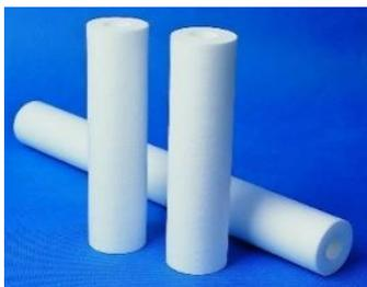
Polypropylene melt-blown filters are the "in-depth" filters; they capture particles throughout the entire filter depth, resulting in an exceptional high retention capacity, conferring on them a longer lifespan hence fewer changeouts which renders these filters more economical. High filtration rates along with low pressure drops make these filters a perfect choice for pre-filtration in water treatment or membrane filtration.
